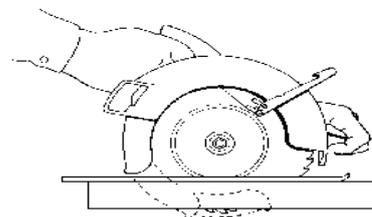
Safety guards must never be removed when a tool is being used. For example, portable circular saws must be equipped with guards. An upper guard must cover the entire blade of the saw. A retractable lower guard must cover the teeth of the saw, except when it makes contact with the work material. The lower guard must automatically return to the covering position when the tool is withdrawn from the work.
