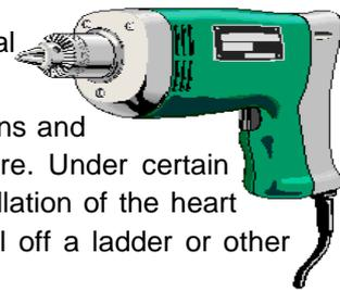
To protect the user from shock, tools must either have a three-core cord with ground and be grounded, or be powered by a low-voltage isolation transformer. Three-core cords contain two current-carrying conductors and a grounding conductor. One end of the grounding conductor connects to the tool's metal housing. The other end is grounded through a prong on the plug. Anytime an adapter is used to accommodate a two-hole receptacle, the adapter wire must be attached to a known ground.
